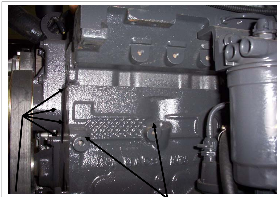
Four M8 mount holes on the front of the engine
