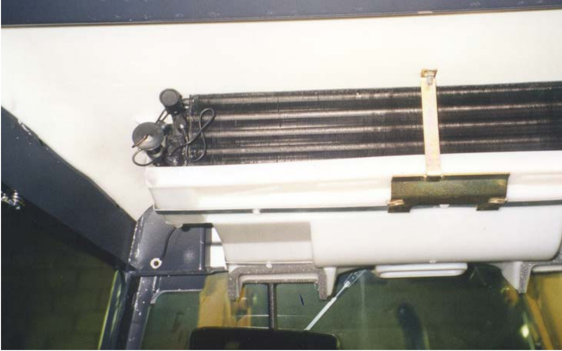
Fitting end of evaporator (left end).
