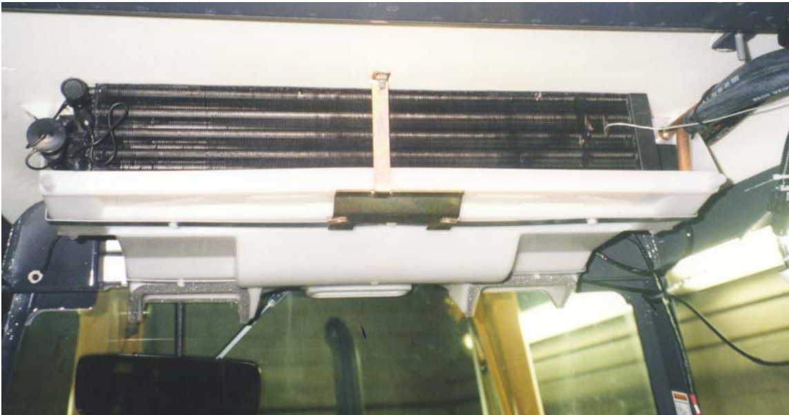
Evaporator mounted in position.
